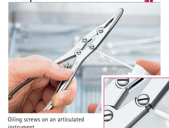
Oiling screws on an articulated instrument
