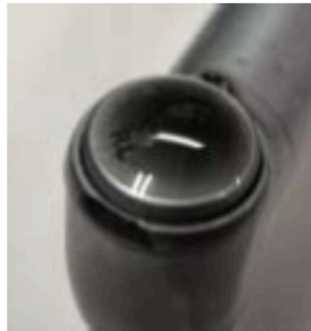
Debris leaking from an unclean chuck during maintenance.
